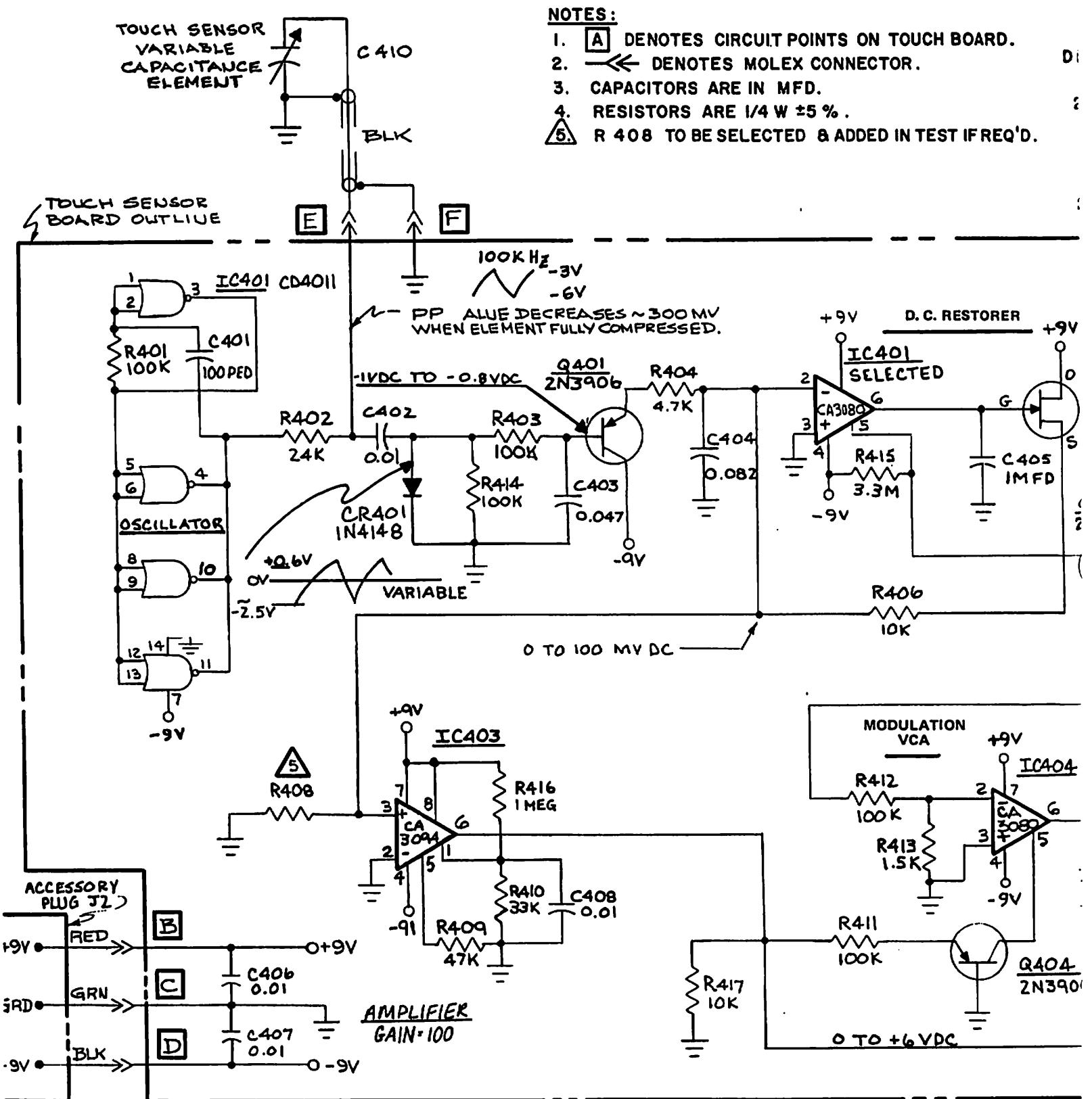
FIGURE 10-4 MINITMOOG TOUCH SENSOR BOARD ASSEMBLY NO. 4 SCHEMATIC DIAGRAM
