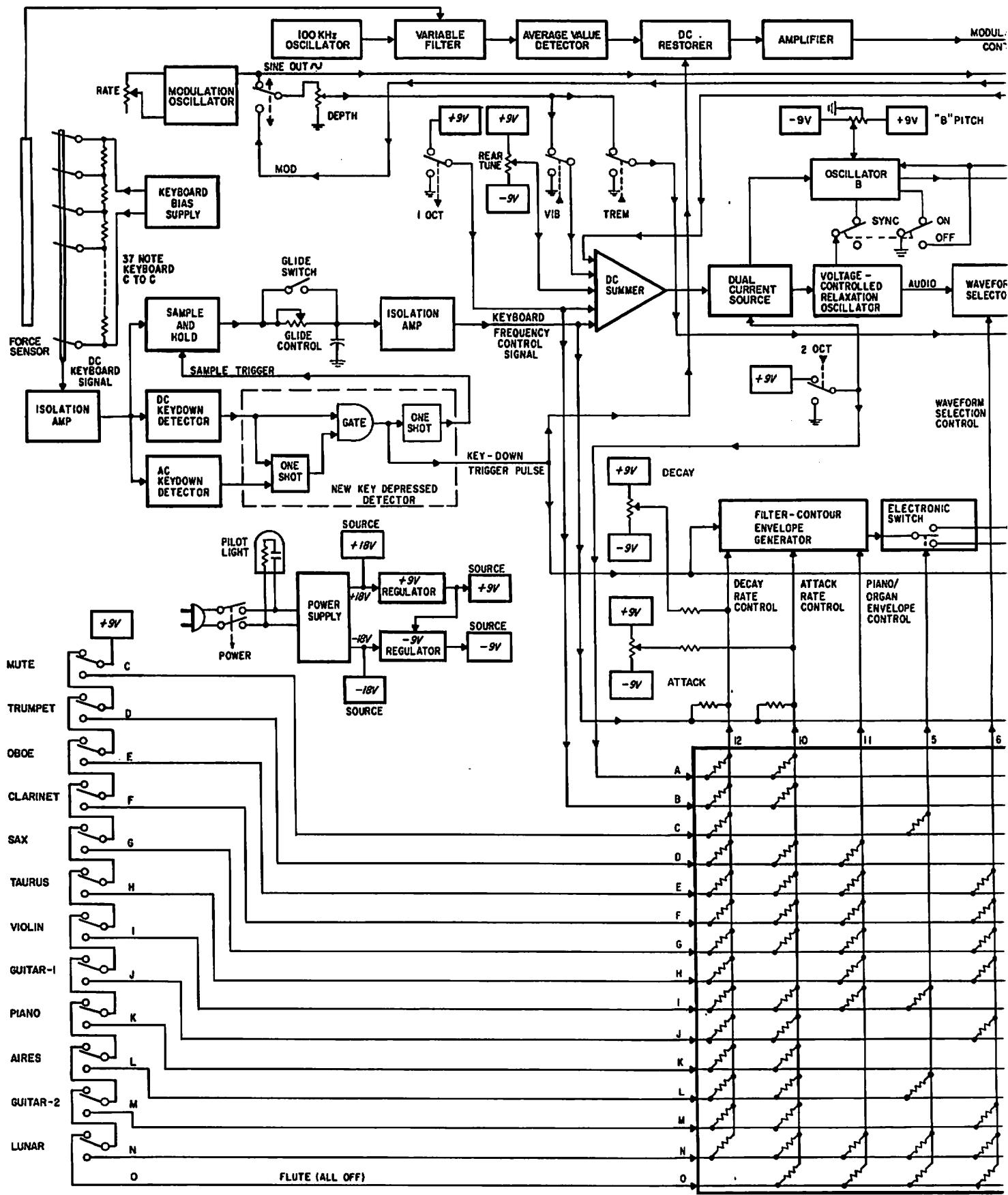
FIGURE 10-2 MINITMOOG BLOCK DIAGRAM
