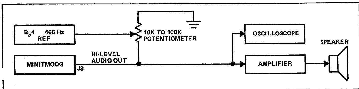
FIGURE 4-1 MINIMAL TEST SETUP FOR TUNING
