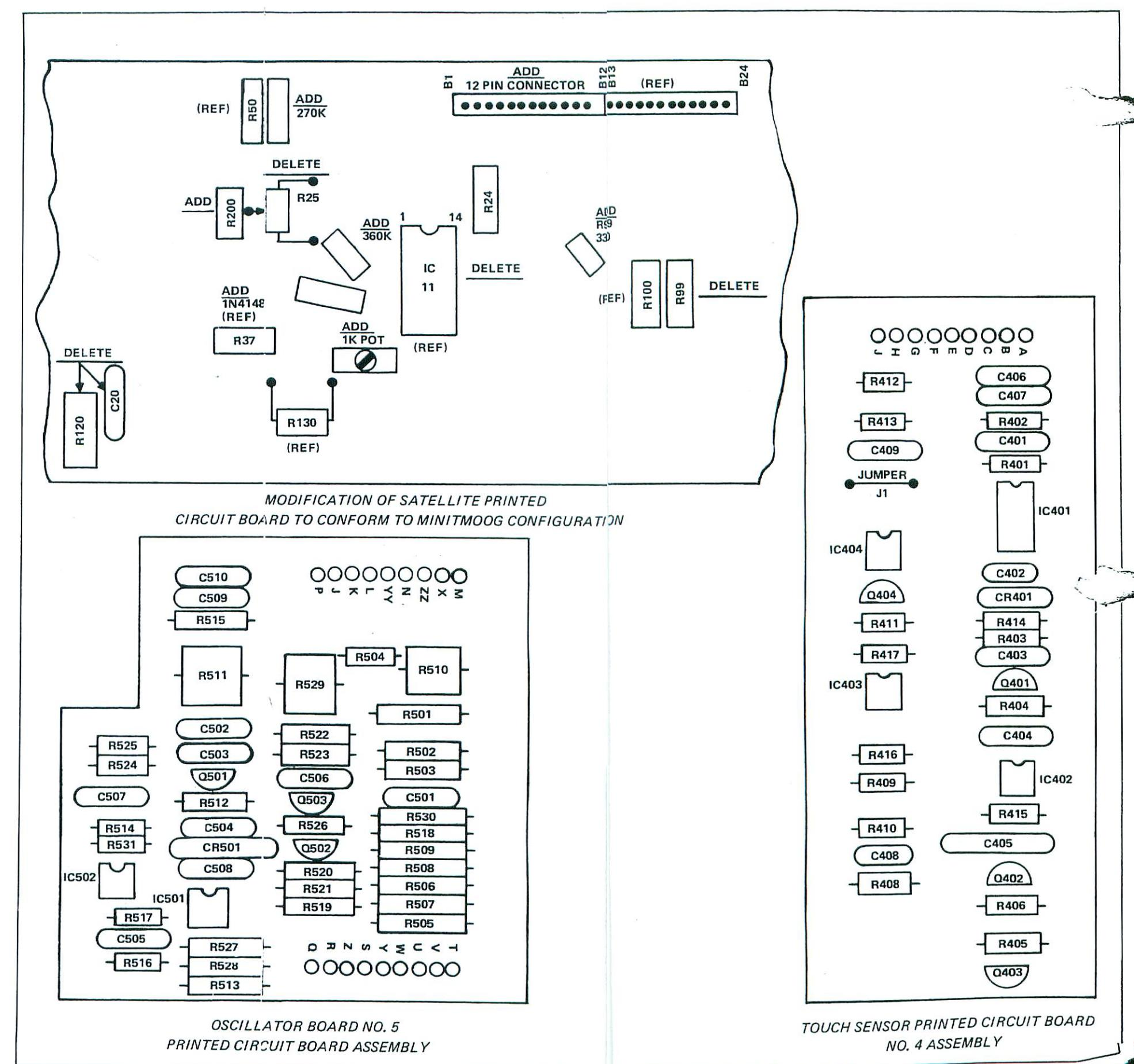
FIGURE 10-3 MINITMOOG PRINTED CIRCUIT BOARD ASSEMBLIES
