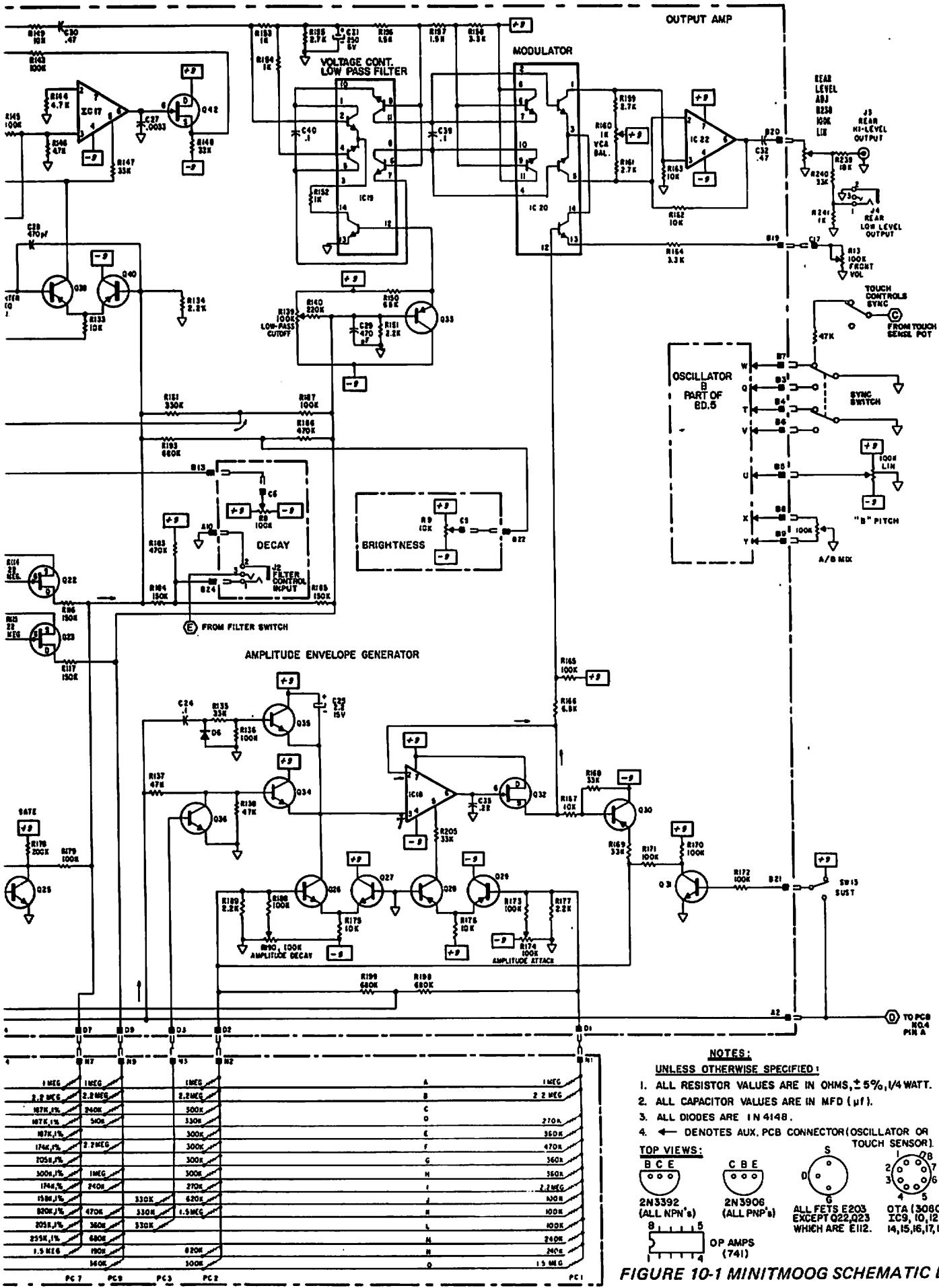
**FIGURE 10-1 MINIMOOG SCHEMATIC DIAGRAM**
