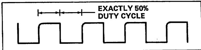
FIGURE 4-6 SQUARE WAVE AT JUNCTION OF R44 AND R119
