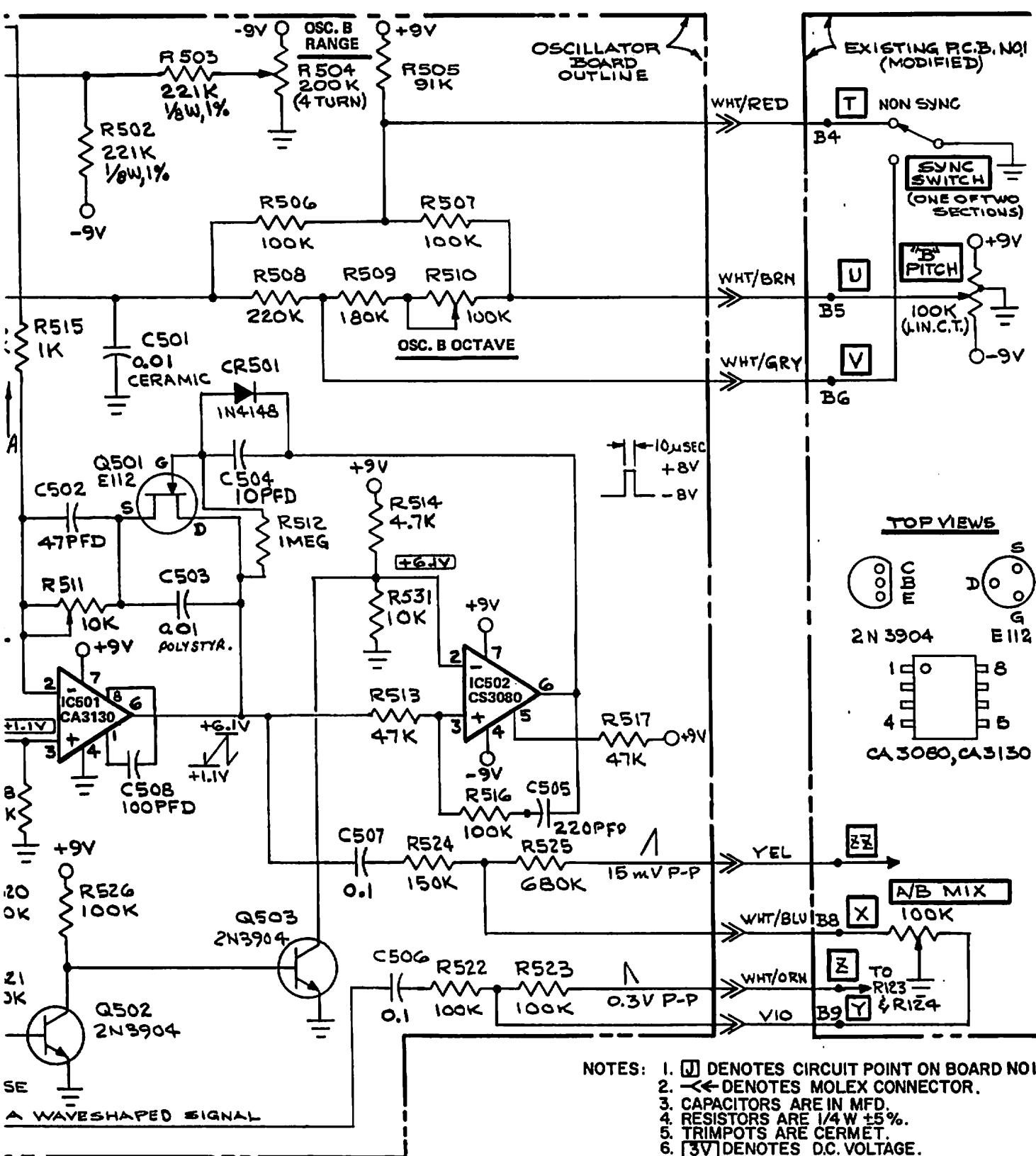
FIGURE 10-5 MINITMOOG OSCILLATOR BOARD ASSEMBLY NO. 5 SCHEMATIC DIAGRAM
