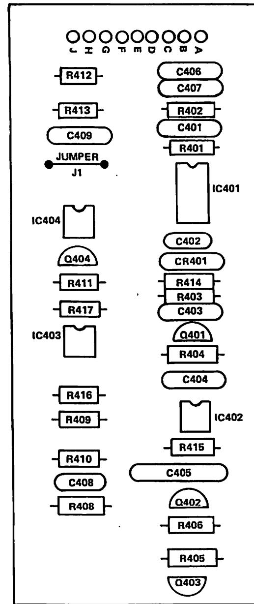
**TOUCH SENSOR PRINTED CIRCUIT BOARD
