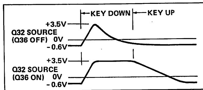
FIGURE 2-5 Source Voltage of Q32
